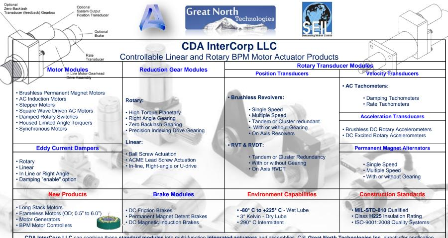
CDA InterCorp LLC can combine these standard modules into multi-function integrated actuators and assemblies. Call Great North Technologies Inc. directly for application engineering assistance or to request a complete set of engineering reference data brochures. Contact Craig Belanger at 514-620-3724 or send us an email at <a href="mailto:craig@greatnorthtech.com">craig@greatnorthtech.com</a>
