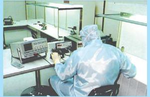
Rotary Accelerometer Testing
