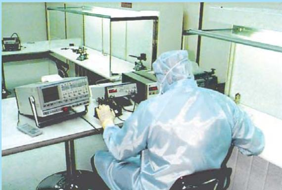
Rotary Accelerometer Testing
